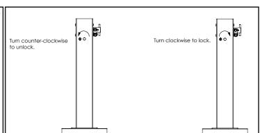
Assemble and install the shaft adaptor and handle as shown in the diagram adjacent here.
