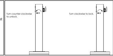
The range of movement is preset ex-factory, but if you find it necessary to fine adjust the ends of travel positions, then extend or retract the length of the stopper bolt as needed.
