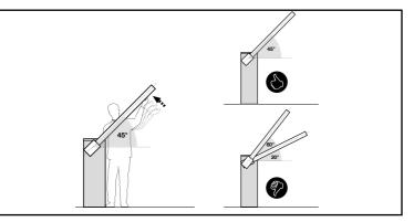
If the spring tension need to be adjusted begin by raising the boom to the full upright position and then locking it in position using the keyed locking mechanism.
