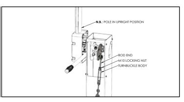
When you are satisfied that the counter balance spring is adjusted correctly to balance the load of the boom pole, make sure the barrier is free to move by ensuring the keyed locking mechanism is "Unlocked"
