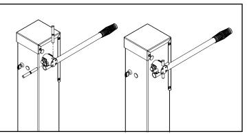
Install and fasten the pole mount base onto the shaft adaptor as shown in the diagram adjacent here.
