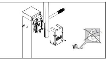
With the boom pole installed and secured in the pole mount clamp, unlock the keyed locking device so that you can check the action of the barrier.
