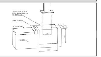
**02.** Using these mounting dimensions, prepare your anchoring points in the properly set and cured plinth.
