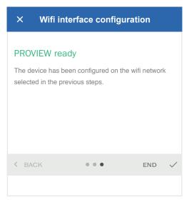
once the procedure terminates, press "END": at this point, it will be possible to manage the various devices connected to the Wi-Fi interface or to the control unit with integrated Wi-Fi.
