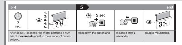
(\*) - IMPORTANT - After programming the option, or after the battery has discharged completely, it is imperative to immediately run 2 complete manoeuvre cycles (up and down = 1 cycle) to activate the function. During this movement, the motor maps the instantaneous load along its travel and automatically sets the maximum sensitivity available with the awning in question.
