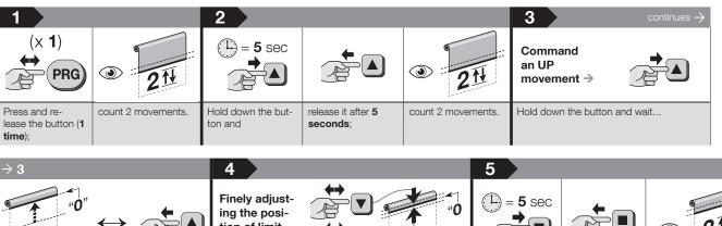
.. release the button as soon as the awning reaches position "0" ( UP limit switch).
