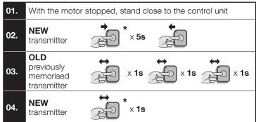
If the procedure terminated successfully the new transmitter is memorised
