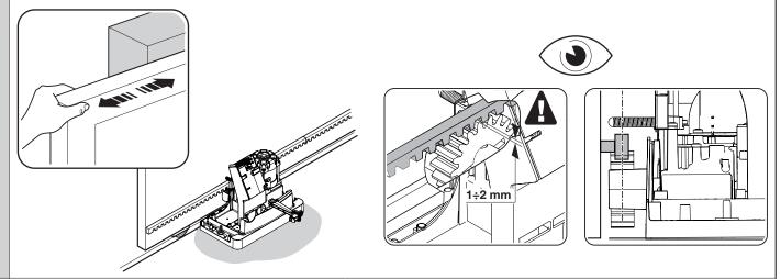
**07.** Vigorously tighten the nuts to fasten the gearmotor to the foundation plate
