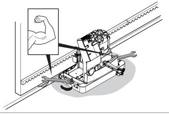
**08.** Install the OPEN and CLOSE limit switch brackets: proceed in the same way for each limit switch
