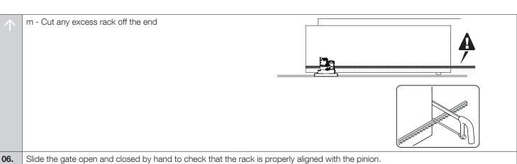
O6. Slide the gate open and closed by hand to check that the rack is properly aligned with the pinion.
