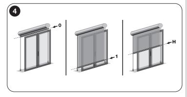
When the limit switches are not programmed yet, the roller shutter can be moved only in the "hold-to-run" mode, i.e. keeping the control key pressed for the desired duration of the manoeuvre; the movement stops as soon as the user releases the key. However, after programming the limit switches, <u>briefly pressing the appropriate key</u> will start the roller shutter and it will stop moving automatically as soon as the roller shutter reaches the required position.
