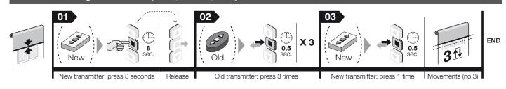
**Note** – When performing the procedures, at any time you can cancel it by keeping the ■ and ▼ keys pressed simultaneously for 4 seconds. Otherwise, do not press any key and wait 60 seconds for the motor to perform 6 movements.
