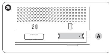
**3.** put the cover of the control unit's containment box back on.
