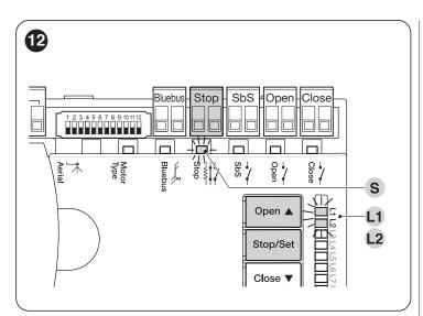
LEDs "L1" and "L2" on the control unit ("*Figure 12*") emit some slow flashes to signal that the learning stage must be carried out.
