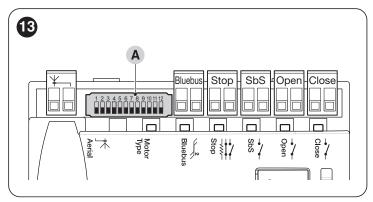
The motor selector must be set before activating the mechanical stop learning function.
