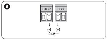
The voltage available at the "SbS" and "STOP" terminals remains even when the "Stand-by" function is enabled on the board.
