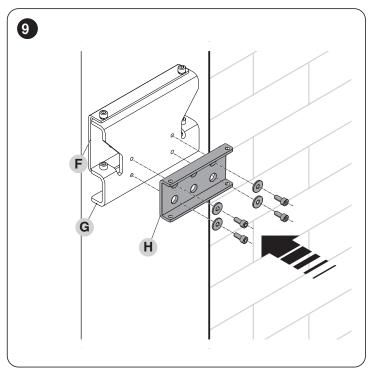
**10.** Fasten the SPOP bracket **(H)** to the adaptation bracket **(G)** making sure that it is aligned with the horizontal axis (*"Figure 11"*).
