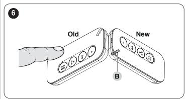
5. On the OLD (Old) transmitter press and slowly release for three times any one of the command keys. With each pressing action, the LED on the NEW (New) transmitter (**B**) switches off and then on again.
