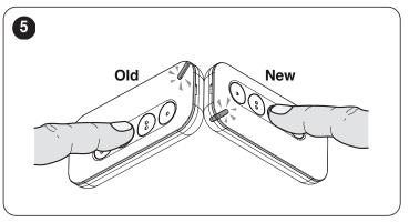
On the OLD (Old) transmitter release the key once the LED on the NEW (New) transmitter (B) lights up steady red.
