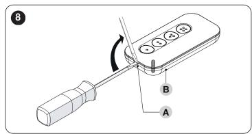
2. press the battery in point (1) and twist the case (B) to release the battery from the clip holding it (2) so that it can be removed
