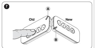
Once the procedure has terminated, the LED of the NEW (New) transmitter (**B**) flashes rapidly to signal the correct transfer of the code.
