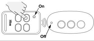
Step 3: When the LED on the new LTX goes off, press and hold the button to copy on the original TX. (TXs must be head to head)
