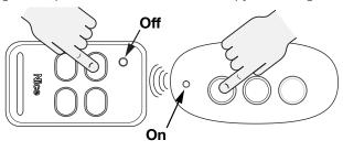
Step 4: Wait for the LED to begin flashing on the new LTX. (+/- 3sec.)
