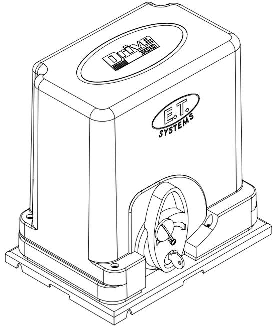
To re-engage the gearbox lower the manual release lever and lock it once again. Gently pull or push the gate by hand until the gears fall into place before triggering the unit to run.
