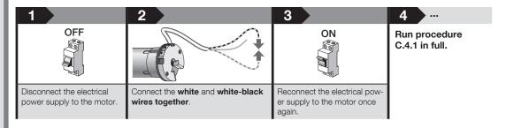
C.4.2.B - Procedure run with a transmitter that has not yet been memorised and the limit switch adjustment buttons on the motor head
