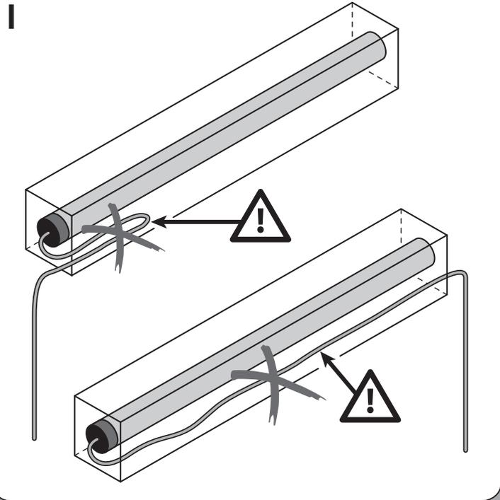
**CAUTION!** - The smaller cables must be handled carefully because they contain very thin wires that could be damaged.
