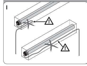
**CAUTION! -** The smaller cables must be handled carefully because they contain very thin wires that could be damaged.
