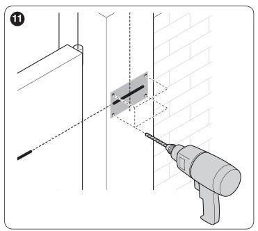
**6.** attach the fixing bracket (**C**) of the gearmotor to the wall using adequate wall plugs, screws and washers (not supplied)
