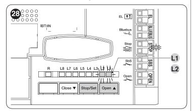
The learning process of connected devices can be repeated at any time, even after the installation (for example, whenever a device must be added); to complete the new learning process, refer to the "*Learning of other devices*" paragraph.
