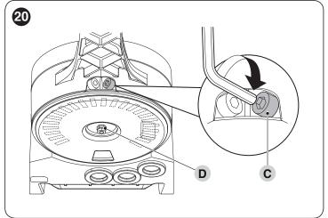
If the system has no closing stop on the ground, the entire procedure must be repeated to adjust the closing limit switch as well
