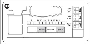
At the end of the learning phase, we recommend letting the control unit run a few opening and closing manoeuvres to verify whether the gate moves correctly and if there are any assembly and adjustment defects.
