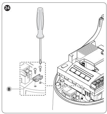
**4.** connect the power cable **(C)** and lock it in place with the cable clamp **(B)**
