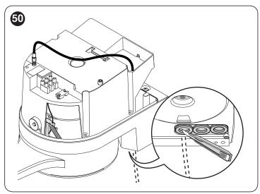
connect the cable to Kio, by referring to the respective instruction manual.
