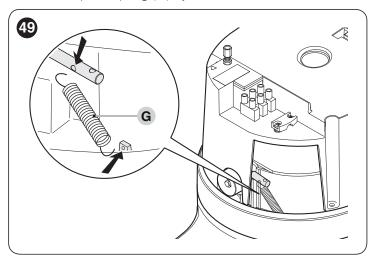
thread the other end of the cable through the hole located on the lower part of the gearmotor
