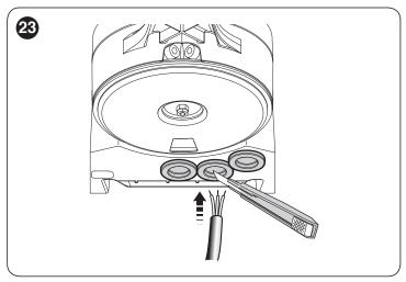
**3.** first connect the motor's power cable with the control unit **HO7124**: loosen the cable clamp (**B**)
