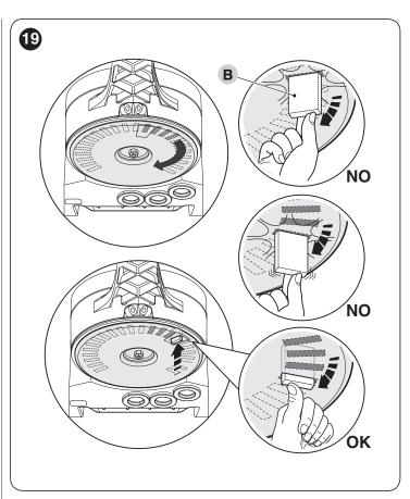
5. turn the disc (A) so that the limit switch does not fall and move the slot towards the position shown in "Figure 18". For a finer adjustment, turn the adjustment screw (C)
