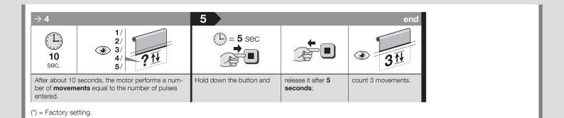
**C**.5 - "FRT" Function: automatic tensioning of the canvas when opening awnings that are not fitted with a mechanism to lock the awning when opening MONO BIDI
