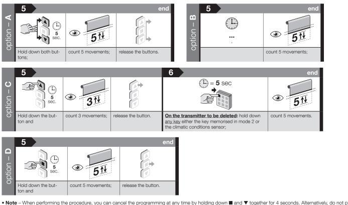
• Note – When performing the procedure, you can cancel the programming at any time by holding down ■ and ▼ together for 4 seconds. Alternatively, do not press any keys and wait 60 seconds for the motor to perform 6 movements.
