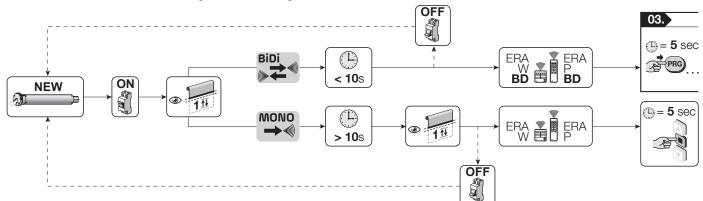
Memorise the first transmitter by performing the procedure described at point A.1 motor configured for ONE-WAY communication, B.1 motor configured for TWO-WAY communication or D.1 motor configured for ONE-WAY communication and OLD generation transmitter lacking the PRG and ESC keys.
