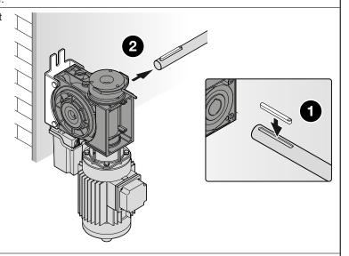
**03.** Fasten the fixing bracket: the gearmotor may be positioned either horizontally or vertically (see pages 3-4). It is important that the roller shaft is horizontal and parallel to the floor.
