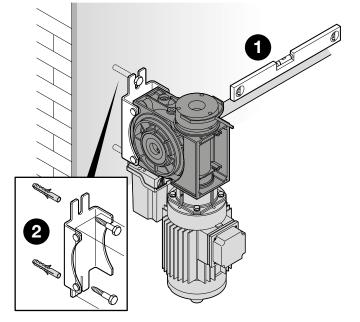
**04.** Ensure the roller shaft cannot shift on its axis: if necessary, use the adjustment systems to block it.
