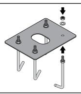
After pouring the concrete into the prepared hole, press the base plate down onto the concrete and ensure the base plate is horizontally level on top of the concrete.
