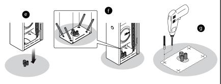
**08.** Place the cabinet onto the anchor bolts and fasten firmly in place. (i)
