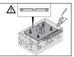
**O5.** Allow sufficient time for the concrete to set and cure before working with the mounting plinth further. Typically this takes about 2 weeks.
